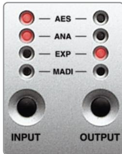
In the example left, the AES and Analogue input groups are both connected to the Expansion Bus output group – the manner in which the AES/EBU and analogue channels are split across the Expansion bus being determined by the setting of the 'connection mode' option switch.
