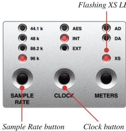
Pressing the Sample Rate and Clock buttons simultaneously will cause the Alpha-Link to display its firmware version number using the top row of meter LEDs until the buttons are released. The unit then returns to normal operation.
